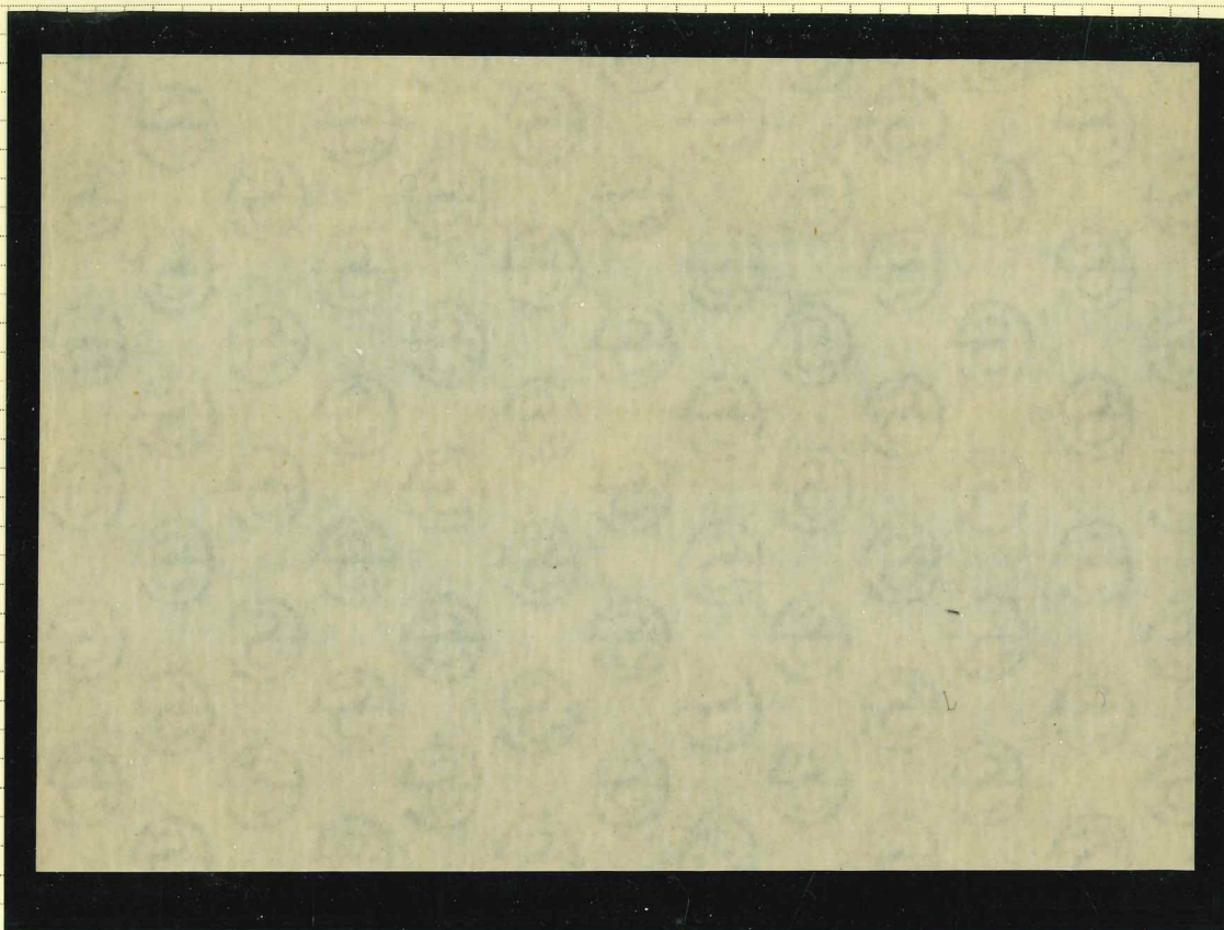
Example of 'Se' Watermarked Paper applied on Mill Paper using the 'Dandy Roll' process 14 x 10 cms
