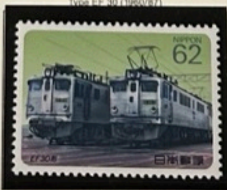
Developed for KANMON under-ocean rail tunnel between Honshu and Kyushu
